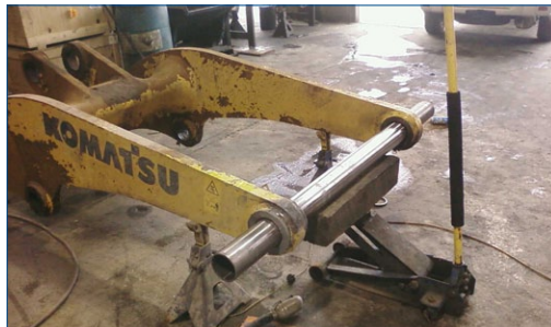
Dummy shaft installed to maintain alignment
