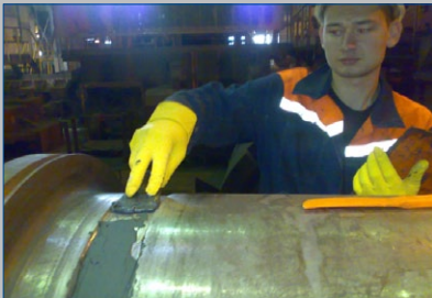
Dummy shaft installed to maintain alignment
