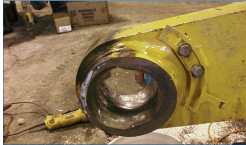
Damaged pin bush housing
